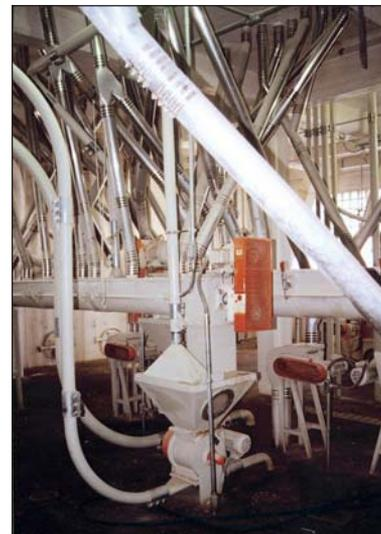
Spouting floor in flour mill featuring a rotary stream splitter dividing product into four Speed Spout outlets.
