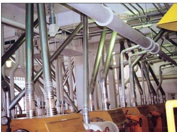
Speed Spout used in spouting and dust control on roll stands.
